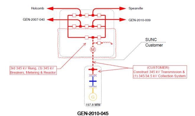
Figure 1. Interconnection Configuration for GEN-2010-045
